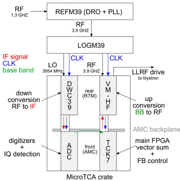
Figure 3: Scheme of the EXFEL 3.9 GHz LLRF signal flow.
