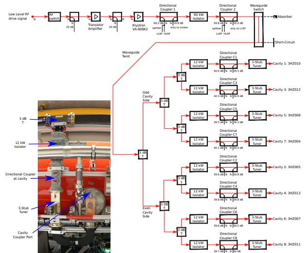
Figure 2: Power RF generation and distribution in AH1.
