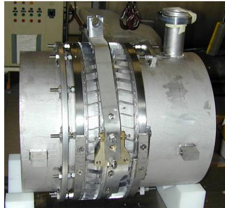
Figure 2: The He-tank and tuner assembly.
