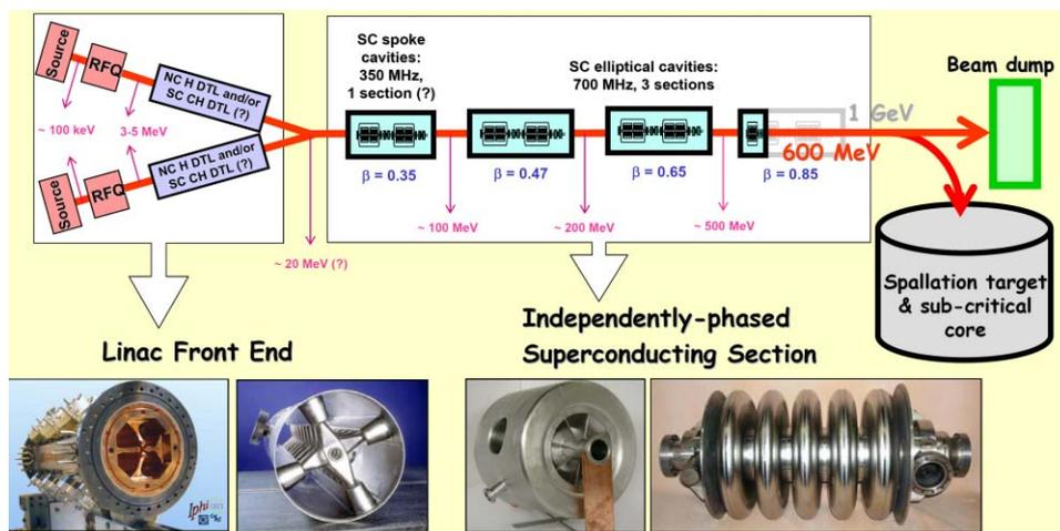
Figure 1: XT-ADS reference accelerator scheme: a doubled linac front end is followed by a fully modular spoke and elliptical cavity SC section, upgradeable from 600 MeV up to 1 GeV for the EFIT needs. Typical cavity prototypes are shown in the lower part: from left to right RFQ, CH structure, Spoke, Elliptical 5-cell.
