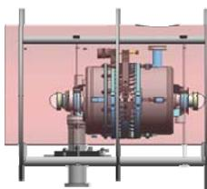
Figure 7: Preassembly of the cavity+coupler in spaceframe.
