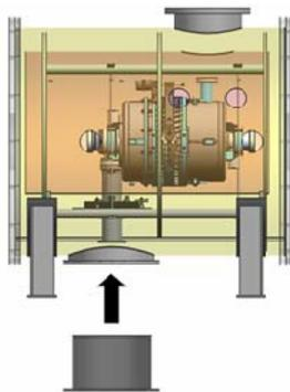
Figure 9: Insertion of the vacuum closure separating the warm coupler window and extension.
