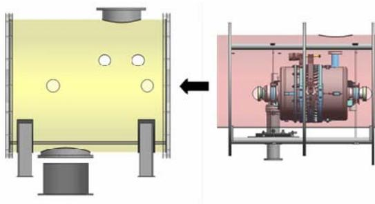
Figure 8: Introduction of the whole cavity + coupler assembly inside the cryostat (horizontal translation).
