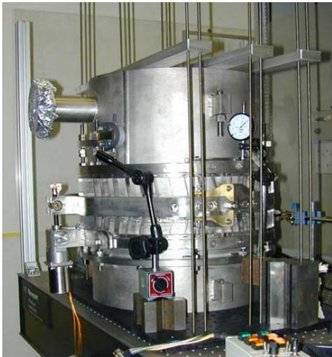
Figure 4: The blade tuner for the TRASCO cavity during mechanical testing at LASA.
