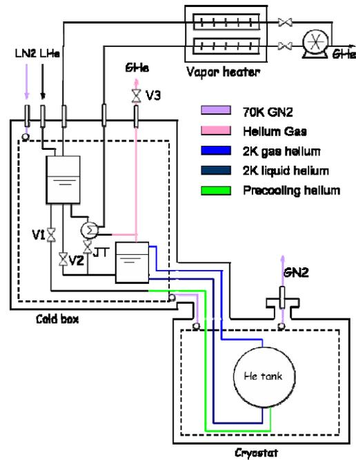
Figure 6: The main cryogenic scheme.
