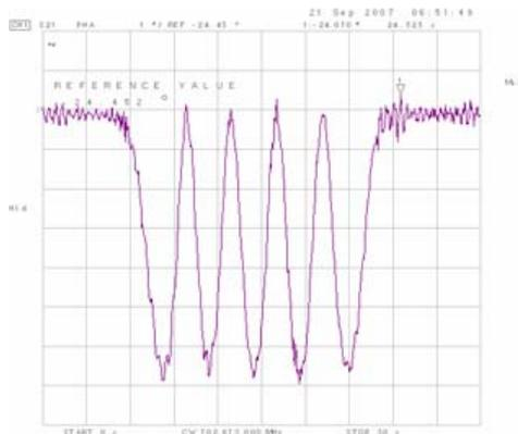
Figure 5: Field flatness profile of the cavity after tuning to the nominal frequency.
