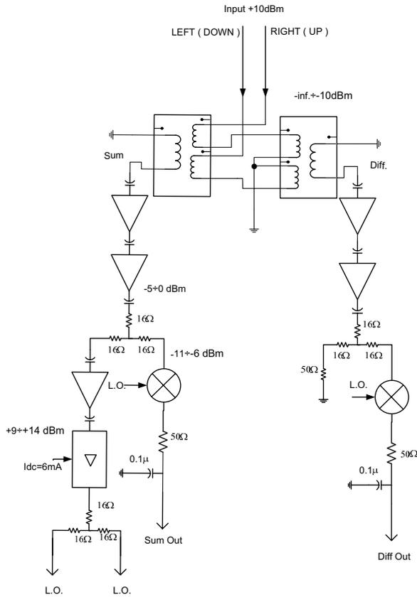
Fig. 2. Conceptual block diagram of the Wire Position Monitor
