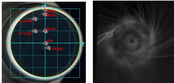
Figure 5: On the left, the plug with regular spot pattern on the surface. On the right, a dark current image showing no hot spots. The dark current value is within usual limits.
