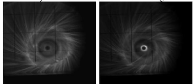
Figure 4: Dark current images from a Mo cathode (#56.2) on the left, and a  $\text{Cs}_2\text{Te}$  cathode (#54.2) on the right. Clear flares are visible as well as three circular regions of different intensities on both cathodes.
