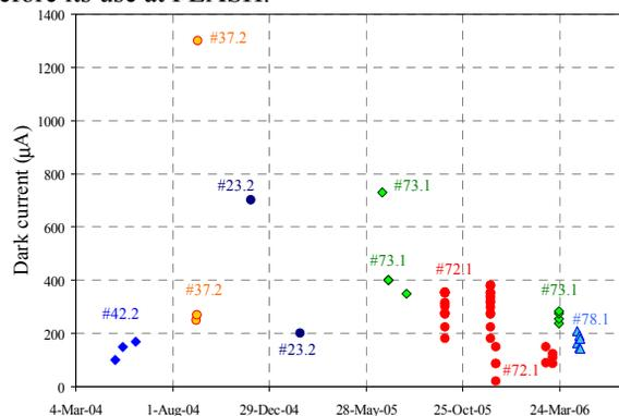
Figure 2: Dark current measurements at FLASH with PITZ-G2 gun, from 2004. Only  $\text{Cs}_2\text{Te}$  cathodes have been used.
