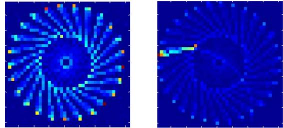
Figure 6: Simulation of the dark current pattern. Left, particles generated on the plug border at 25 angles. Right, one “hot spot” on the plug border has been enhanced.
