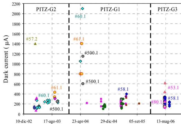
Figure 1: Dark current measurements at PITZ starting in '02 till today. Three different guns are considered. Data from  $\text{Cs}_2\text{Te}$  and Mo cathode are reported.
