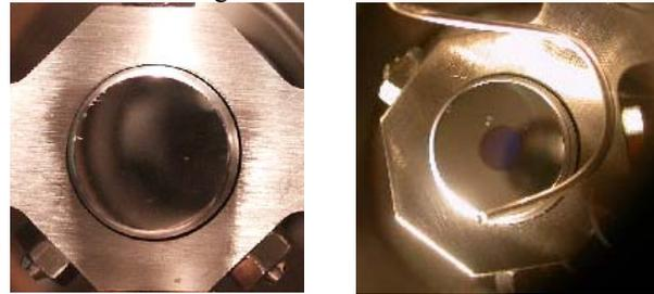
Figure 3: Left: Cathode #53.1 with scratches on the border. Right: A picture of cathode #37.2 taken after the accident: near the coating a bright particle is visible.
