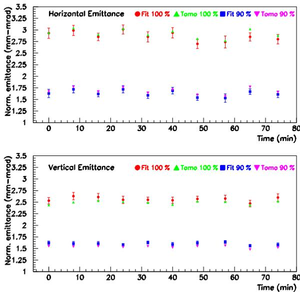
Figure 3: Transverse rms emittance measured at 127 MeV for a bunch charge of 1 nC repeated several times within 75 min.[13] Horizontal and vertical projected emittances are shown analyzed with two different methods (see [14] for details): the true rms calculated from the full and from 90 % of the intensity, and calculated using a tomographic technique.
