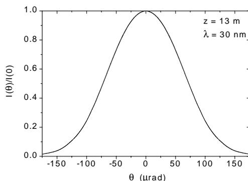
Figure 3: Simulated intensity distribution of the FEL radiation in the far zone.[11] The angular divergence is  $150 \mu\text{rad}$  (fwhm) in good agreement with the measurement.
