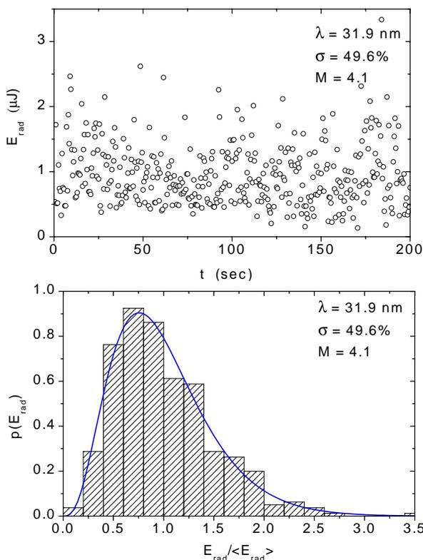
Figure 4: Example of the measured energy in the FEL radiation pulses for a certain period of time (top). The same data normalized to the average energy are shown as a histogram giving the probability distribution (bottom).[10] The rms energy fluctuation  $\sigma$  of 49.6% gives the number of lasing modes  $M$  of 4.1, which determines the Gamma-distribution drawn as a solid line. (The data bins are scaled such that the area is equal to the integrated Gamma-distribution.)
