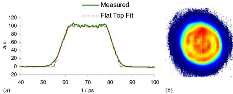
Fig. 2. (a) Temporal profile of the laser micro pulse measured at a wavelength of 524 nm using a streak camera. Ten laser pulses have been integrated. The dashed line shows a flat top fit with  $\sim 24$  ps FWHM and 6 ps rise/fall time. (b) Transverse laser intensity distribution on the virtual cathode. Modulation depth  $\sim 20\%$ .
