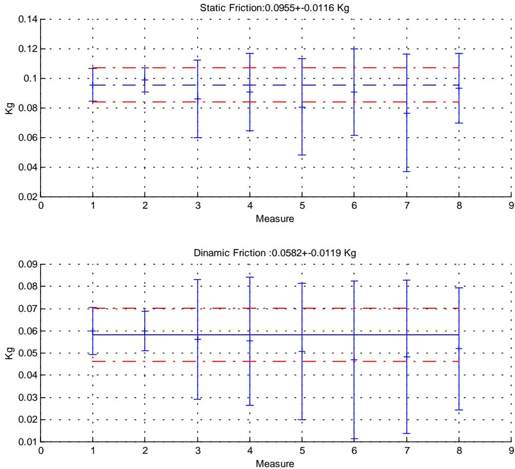
**Figure 6.** Results summary prepared by the “Data Analysis Tool”. Results from the eight measures (four movement patterns, two run for each trip) are compared to achieve a final result value (and error) for dynamic and static friction.
