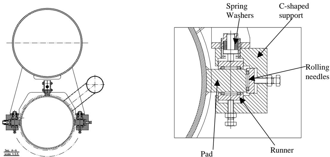
**Figure 1.** The cavity support scheme. Each cavity is attached to the HeGRP by means of four fixtures. Each fixture includes rollers, runners and reference screws to define the vertical and lateral position. Spring washers are used to give a constant  $80 \text{ kg}_f$  load. Rolling needles keep the cavity longitudinal position free.
