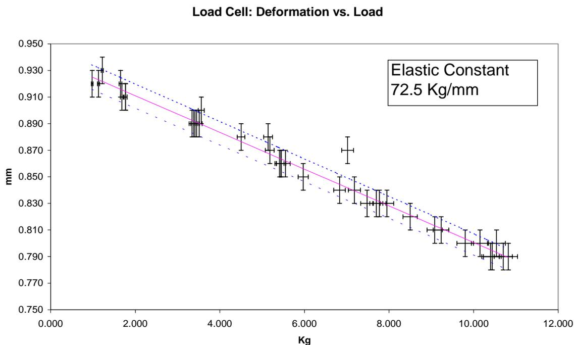
**Figure 3.** Displacement vs. force characterization of the load cell. The device shows a good linearity and reproducibility, with an elastic constant of 72.5 kg<sub>f</sub>/mm.
