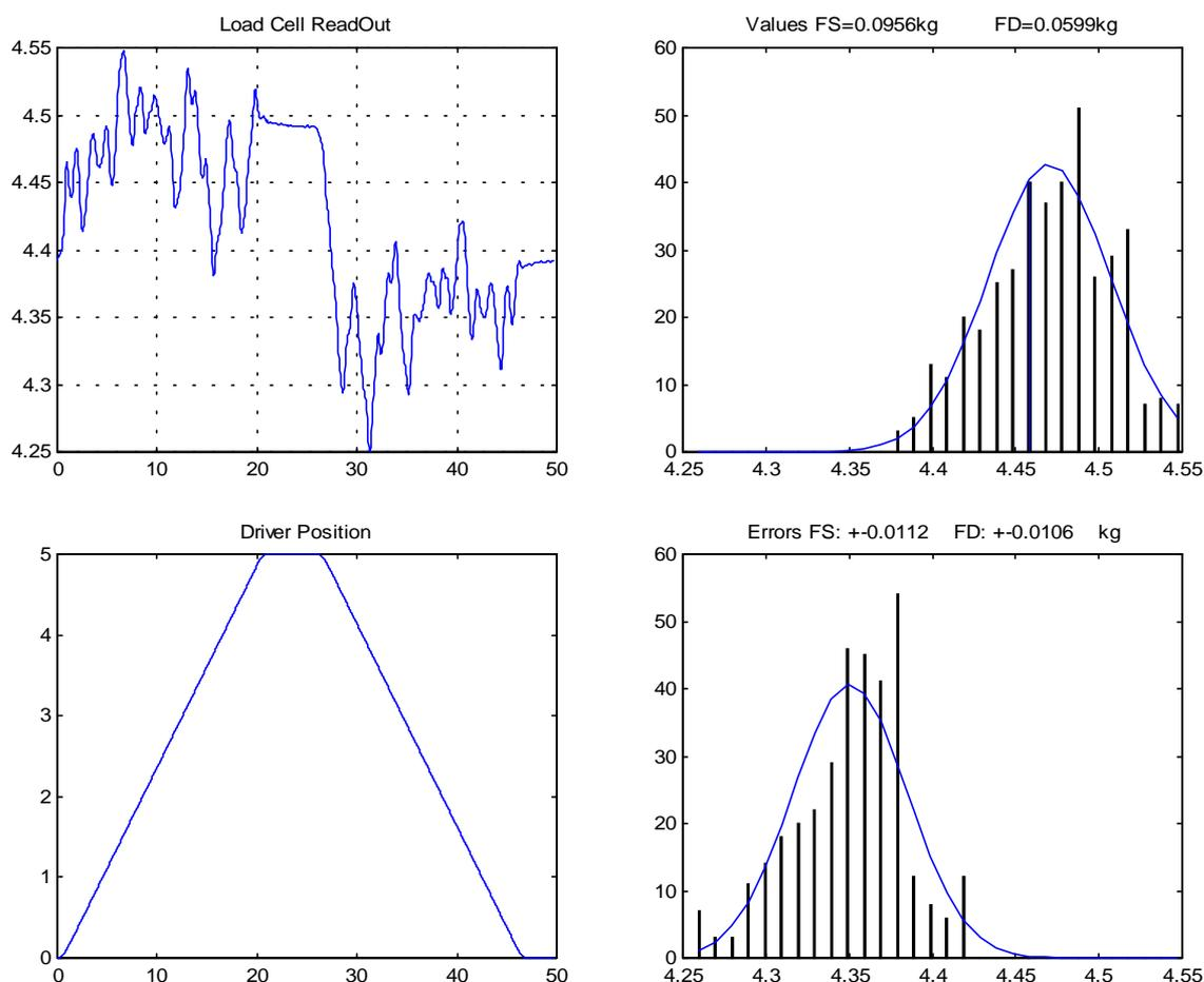
**Figure 5.** Data as output by the “Data Analysis Tool” developed to analyze the friction system results, for the case of the movement pattern of type I (Slow motion and single step). Studying the Load Cell tracks and checking them with the driving motor data the oscillations predicted by friction theory are reconstructed, and static and dynamic friction are evaluated, with their errors.
