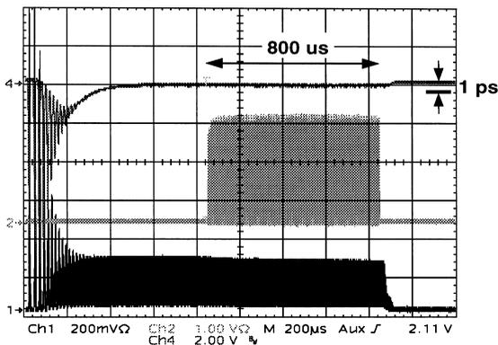
Fig. 2. Oscilloscope trace of the output of the pulse train oscillator (PTO) (trace 1), the phase of the pulses relative to the reference (trace 4), and the pulse train after amplification measured in the green with a fast photodiode (trace 2). Note, that due to the scale (200  $\mu$ s per div.) individual pulses in the train are not visible. Indicated is the vertical scale of the phase signal corresponding to a phase shift of  $0.5^\circ$  of 1.3 GHz, which corresponds to 1 ps.
