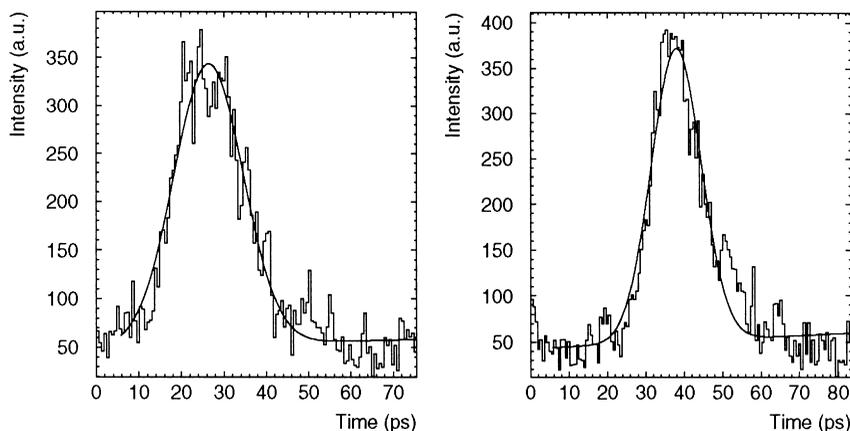
Fig. 3. Two examples of laser pulse shapes measured with a streak camera at 262 nm. The pulse length determined by a fit to a Gaussian profile is  $\sigma_t = 6.3 \pm 0.6$  and  $8.0 \pm 0.1$  ps, respectively.
