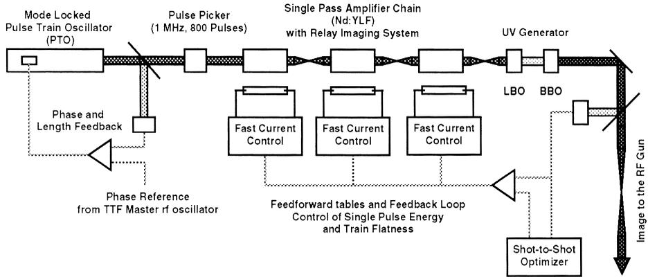
Fig. 1. Schematic overview of the TTF photoinjector laser system.
