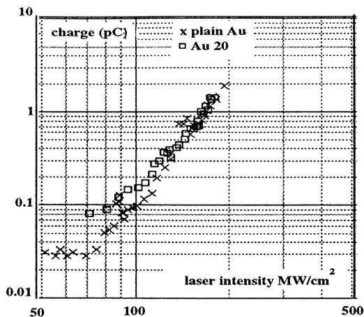
Fig. 1. Charge emitted versus energy of the laser pulse obtained with a cathode of plain gold (◇) and gold coated with a 20 nm film of nanostructured carbon (+). The slope in log-log diagram results in 4.3.
