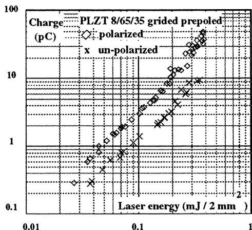
Fig. 2. Emitted charge versus laser energy for PLZT 8/65/35 illuminated with violet light in log-log plot. The slope of the line is 2, for  $Q \propto I^2$ .
