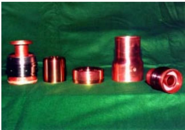
Fig.8 - Parts of the disassembled coupler.
