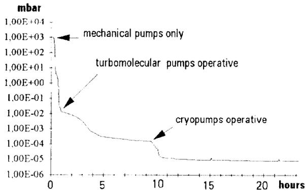
Figure 2. Pressure Vs time of a typical pumpdown
