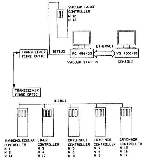
Figure 6. Architecture of the vacuum control system
