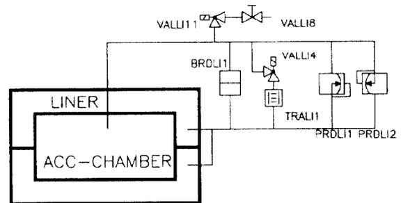
Figure 4. Schematic layout of the safety and balance system
