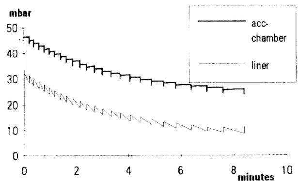
Figure 5. Acceleration chamber and liner pressure Vs time
