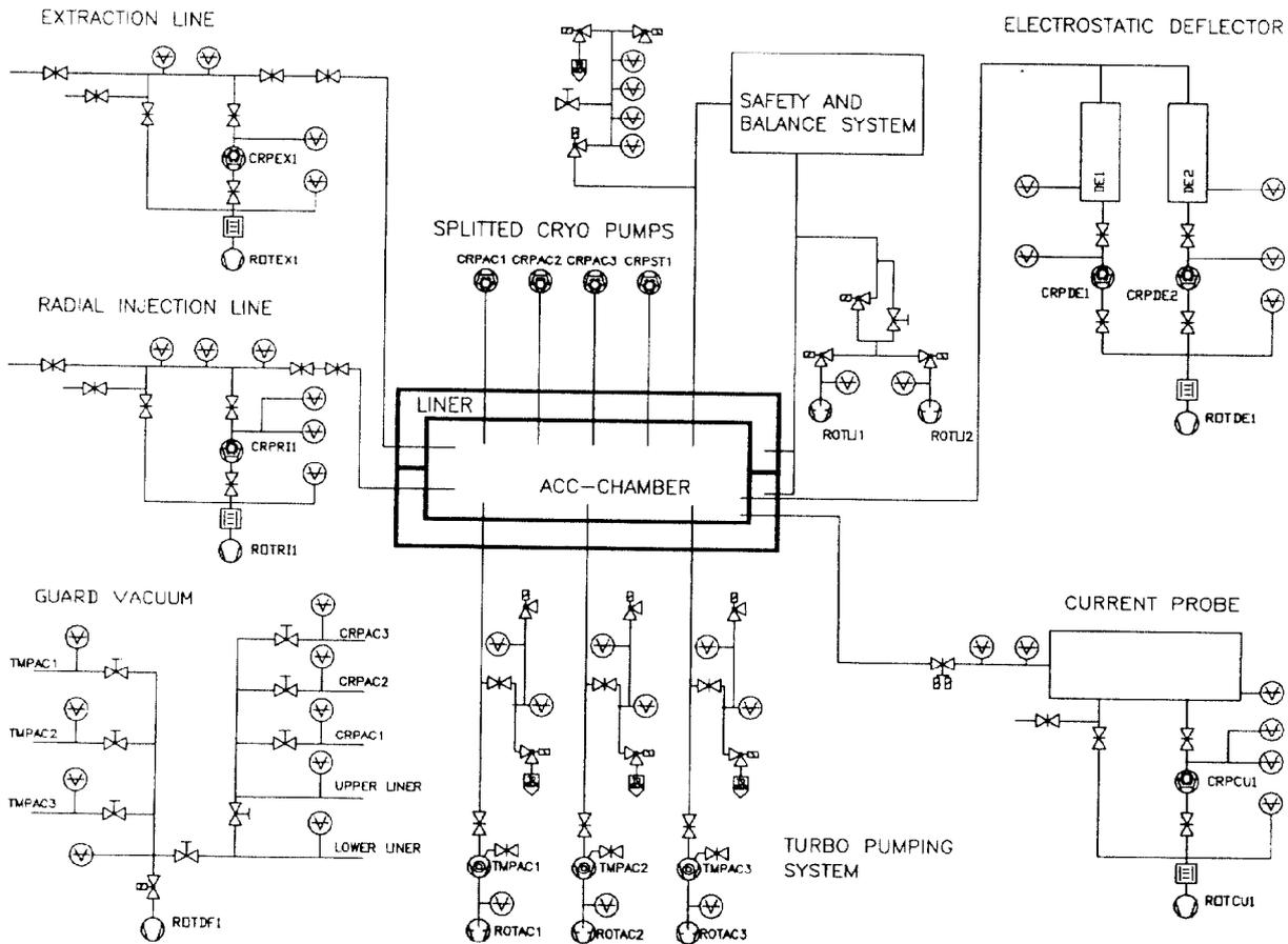
Figure 1. Schematic layout of the vacuum system.
