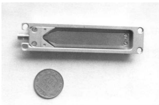
Fig. 1. Photograph of a phase probe.
