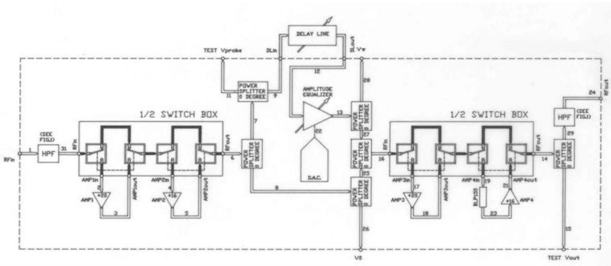
Fig.4. Filtering section scheme
