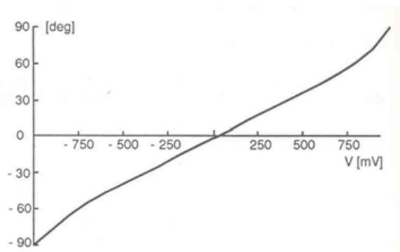
Fig.9 Phase detection system output .This graph is obtained after phase detector output signal processing.
