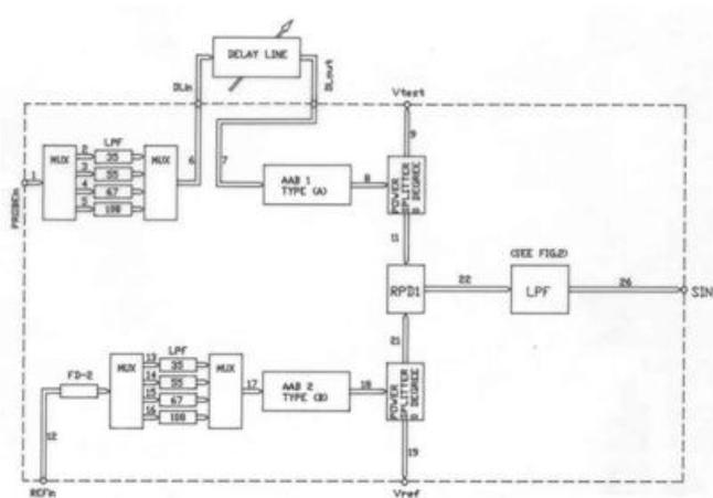
Fig.5 Phase detection system. The frequency doubling system is also shown.
