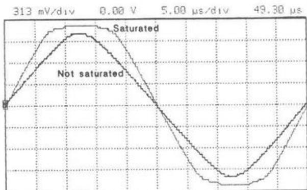
Fig.6 Phase detector output characteristics, taken from a HP 54201A/D digitizing oscilloscope.
