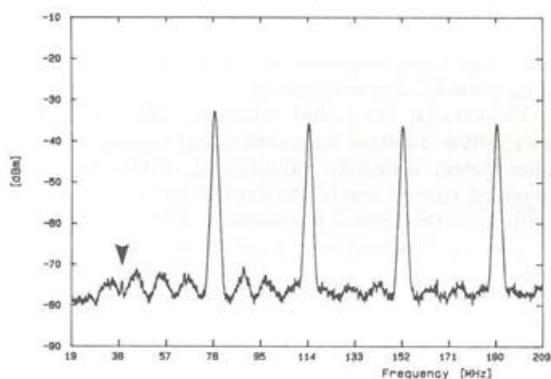
Fig.8. Signal after interference filter. The arrow show 1<sup>st</sup> harmonic power level.
